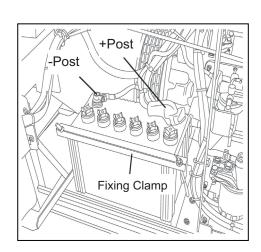
Reinstall a new battery in the reverse order (always install the cable to the positive (+) post of the new battery first).
