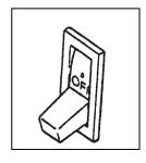
By turning this circuit breaker on the control panel to ON, Power will be transferred to the output receptacles and to the load side.
