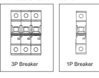
Each receptacle, 3-Phase and 1-Phase is incorporated with circuit breaker respectively. The breaker trips on overload or short-circuit on to stop power transmission to load.
